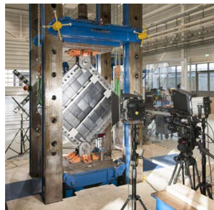
Avery with rectangular shear frame, video, online monitoring, DIC,
