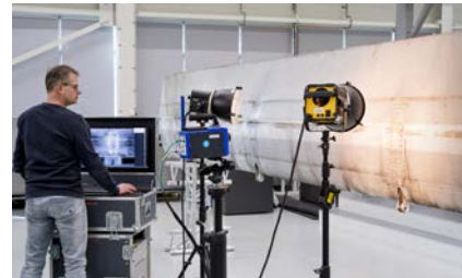
Thermography on wing flap
