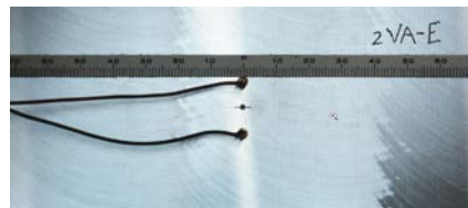
Fully automated crack growth monitoring
