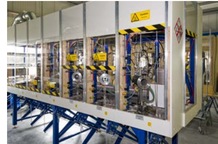
Creep frames combined within a controlled environmental cabinet
