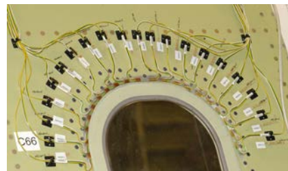
Strain gauges on window panel
