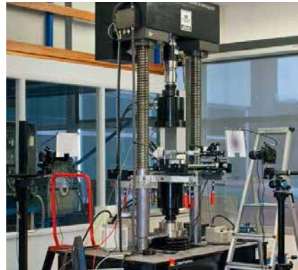
Amsler, crack growth sample, see below
