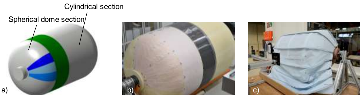
Figure 1: a) CAD Model of booster demonstrator; b) Application of auxiliary material packages on full-scale demonstrator; c) Application of VAP membrane on model (scale: 1:6)
