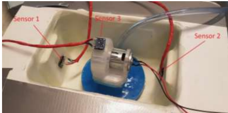
Figure 2: Prototype actuator for automated mould release
