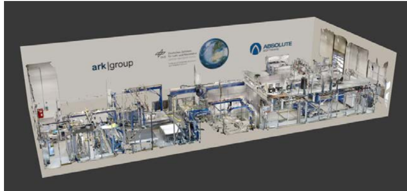
Figure 1: Digital Twin of RTM production line "Evo"
