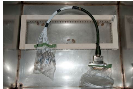
Cables inside fluid susceptibility cabinet
