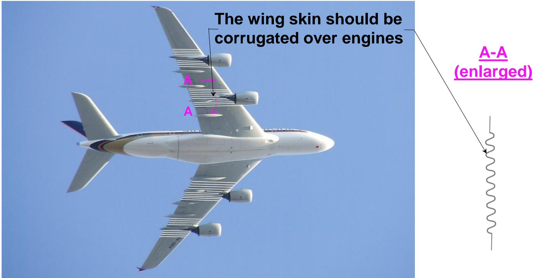
Fig. 2-Aircraft with corrugated wing skin on pressure side, over engines
