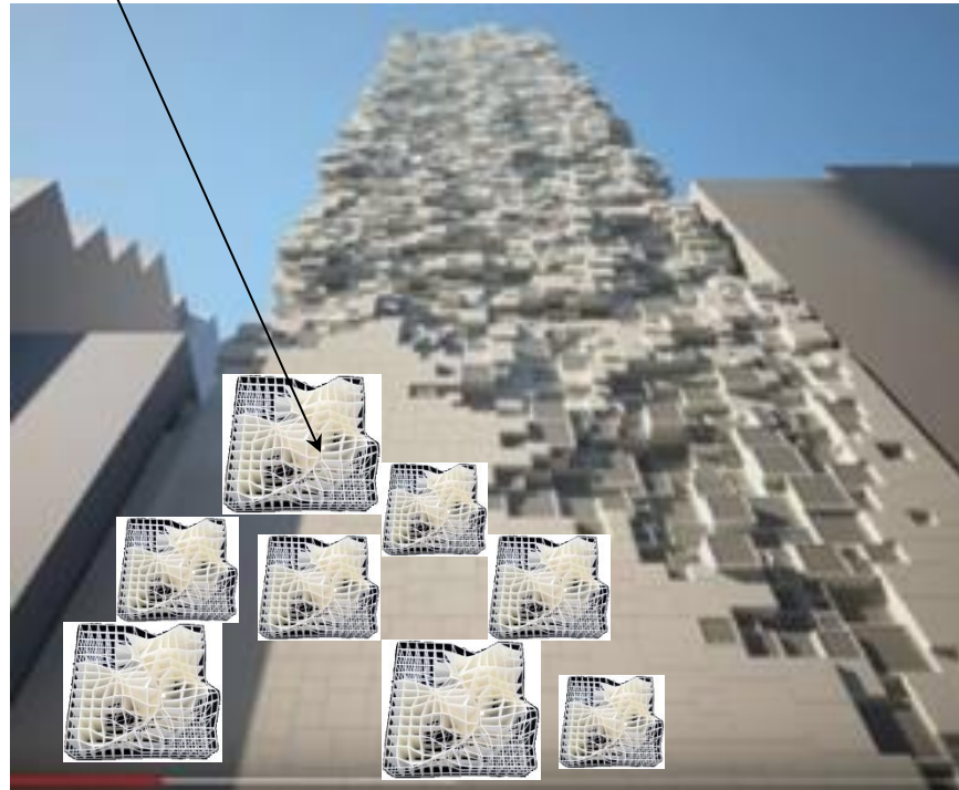
Fig.9- Lining of buildings' exterior with Schroeder type structures for noise diffusing
