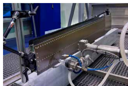
Squirter inspection large aircraft component
