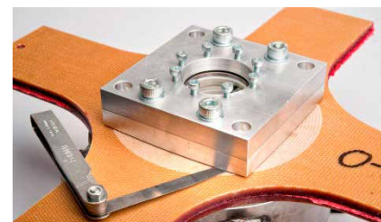
Transparent Anti Buckling Guide for Biax
