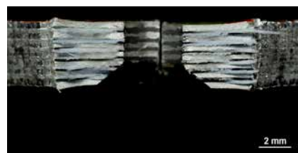
Fracture surface of glare skin
