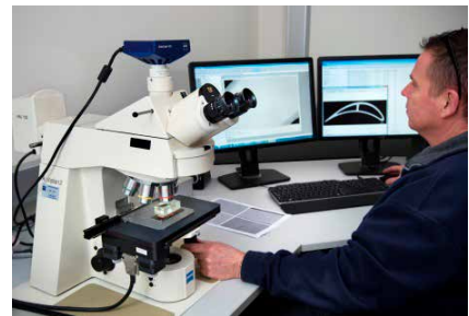
Light microscope for material characterization
