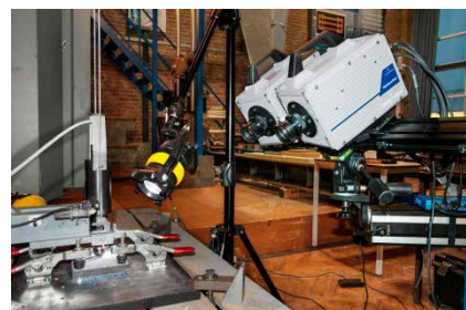
Droptower with High Speed DIC instrumentation
