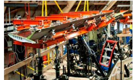
Dassault F5X Stabilizer and elevator loading with variable elevator deployment
