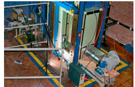
Avery with environmental cabinet (80°C), video, DIC and high speed camera
