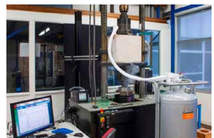
24/7 full spectrum fatigue testing at -55 °C
