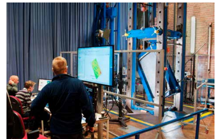
Avery with rectangular shear frame, video, online monitoring, DIC, high speed camera
