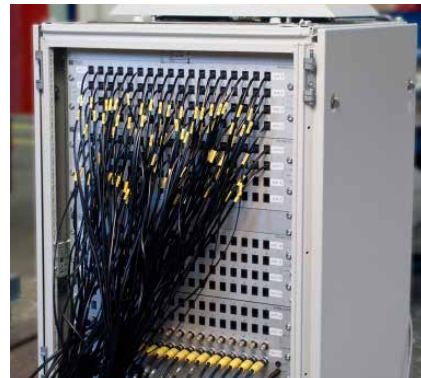
Data Acquisition System (288 channels)
