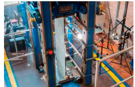
Avery with video, DIC, high speed camera
