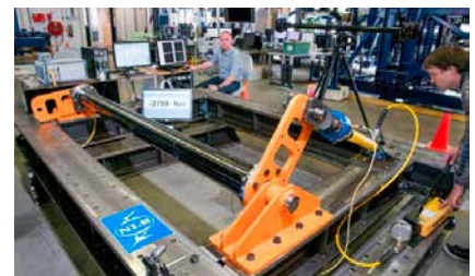
Torsion test using modular setup building elements
