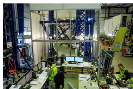
Bombardier C-series flap track testing at -55°C (24/7)
