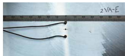
Fully automated crack growth monitoring
