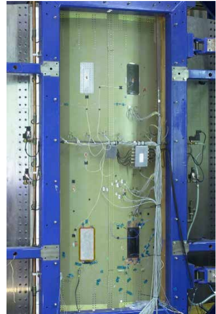
Demonstration of the feasibility of specific SHM systems on a representative structure (Glare fuselage panel with bonded and riveted repair patches)
