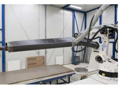
The challenge: to find out whether thermoplastic materials can be used for really thick and large components, for example in aircraft. Parts of the aircraft engine pylon become very hot during normal use of the aircraft. For that reason, the pylons currently used are commonly made of titanium. Most of the parts, such as ribs and spars in the pylon, are made by forging and milling. A reduction of costs might be achievable if the titanium parts can be replaced by composite materials.
