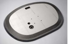
The challenge: to design and manufacture a composite forward pressure bulkhead that is 10% lighter than the original aluminium bulkhead, while still meeting bird impact and stiffness requirements. An obvious job for NLR and partner Airborne, commissioned for Clean Sky Green Regional Aircraft ITD.
