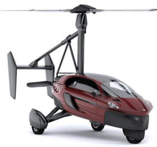
The PAL-V Liberty is a true innovation. This new Personal Air and Land Vehicle is capable of driving on the road at 160 km/hour and of flying at up to 180 km/h. In flying mode, the gyrocopter principles are applied. In drive mode, the rotor and propeller are folded. The foldable rotor blades and foldable propeller have to comply with the EASA CS27 small rotorcraft design principles and airworthiness requirements.
