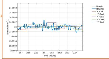
The left figure shows the measured temperatures. The black line indicates the set point temperature, and 'NTCmain' is the controlled chilled water temperature. NTCext1 to NTCext5 indicate 5 external temperatures sensors that are located in the outlet water flow of the chiller. The figure above shows that the temperature of these external sensors is kept within  $\pm 0.0005$ °C temperature stability.
