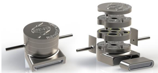
Figure 6: Multi-Parallel Micro-Pump (CAD drawing and picture)
