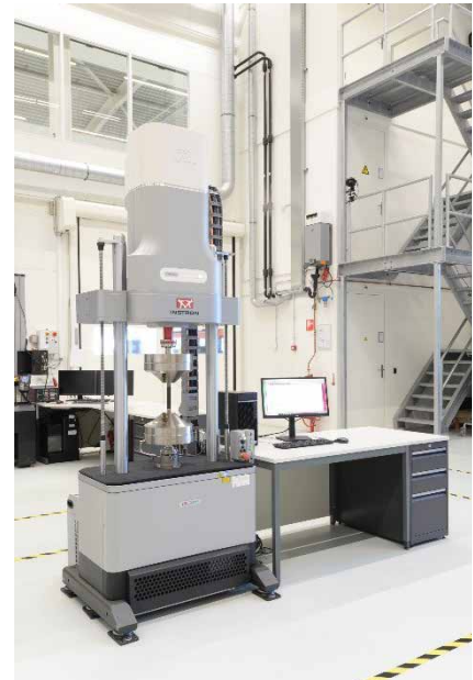
Instron E20000 All Electric dynamic test machine
