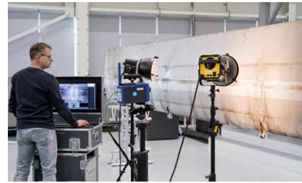
Thermography on wing flap
