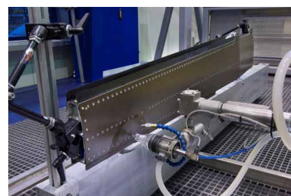
Squirter inspection large aircraft component
