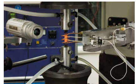
Creep test with coil heating, strain measuring and grip cooling
