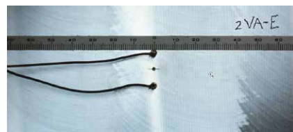
Fully automated crack growth monitoring
