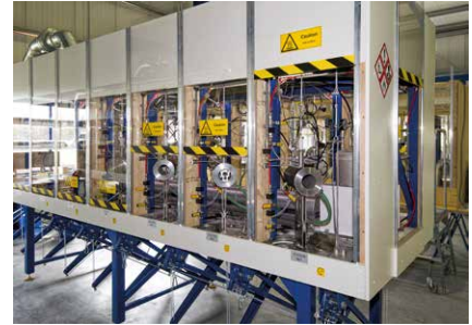
Creep frames combined within an controlled environmental cabinet
