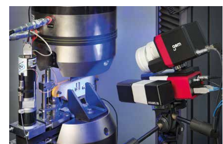
DIC measurement using 6M camera
