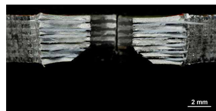
Fracture surface of glare skin
