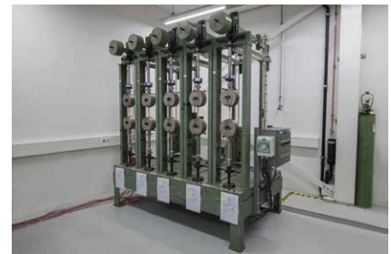
Series of creep frames within a controlled room.
