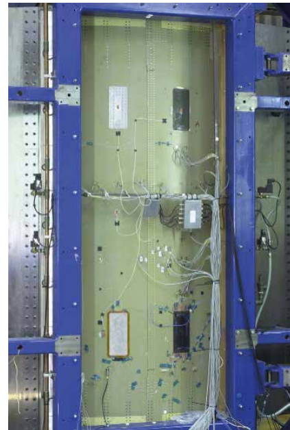
Demonstration of the feasibility of specific SHM systems on a representative structure (Glare fuselage panel with bonded and riveted repair patches)
