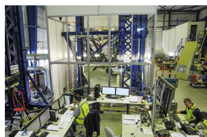
Bombardier C-series flap track testing at -55°C (24/7)
