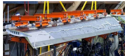
Reflective markers on the elevator surface, recorded by SPR cameras for SPR processing of 3D displacements
