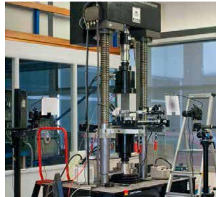
Amsler, crack growth sample, see below
