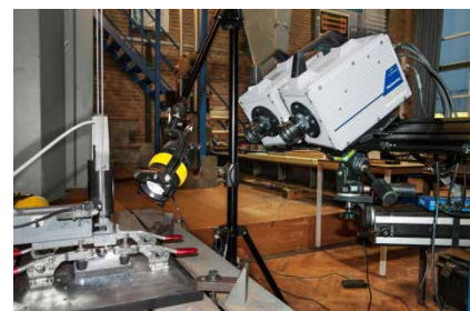
Droptower with High Speed DIC instrumentation
