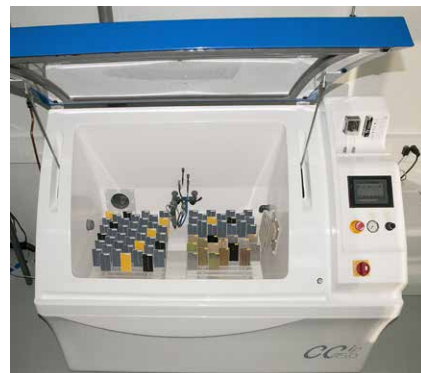
Salt spray cabinet 1
