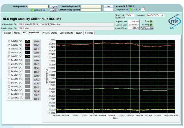
The Graphical Users Interface (GUI) can be opened in a browser on any PC that is connected to the same network as the chiller. The GUI contains displays for all the measured values (temperatures, pressures, volume flow) and is used to control the system. The measured data is automatically stored.
