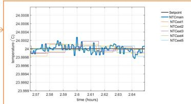
The left figure shows the measured temperatures. The black line indicates the set point temperature, and 'NTCmain' is the controlled chilled water temperature. NTCext1 to NTCext5 indicate 5 external temperatures sensors that are located in the outlet water flow of the chiller. The figure above shows that the temperature of these external sensors is kept within ±0.0005°C temperature stability.
