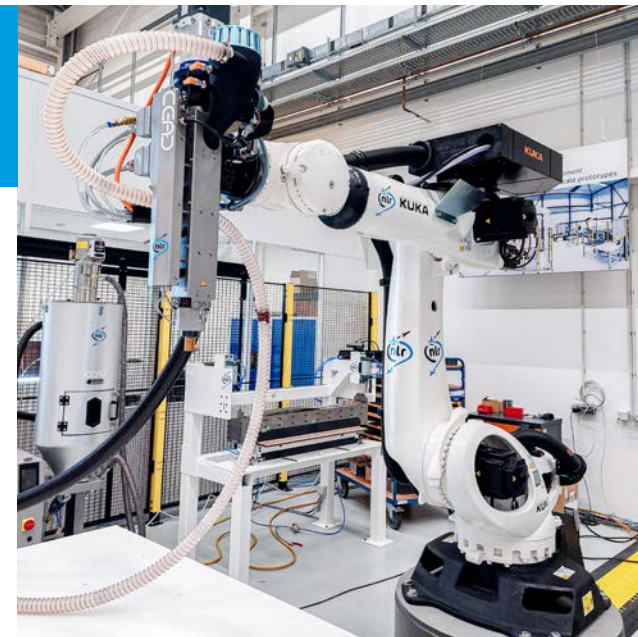
LSAM setup at the NLR: CEAD S25 extruder mounted on KUKA KR240 robot
