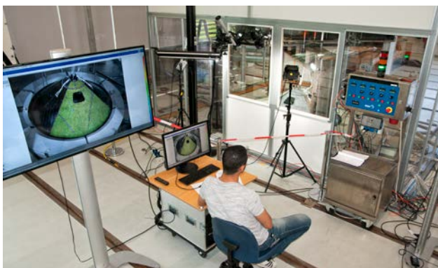
Actual full-scale space structures testing at -180^{\circ}\text{C} .
