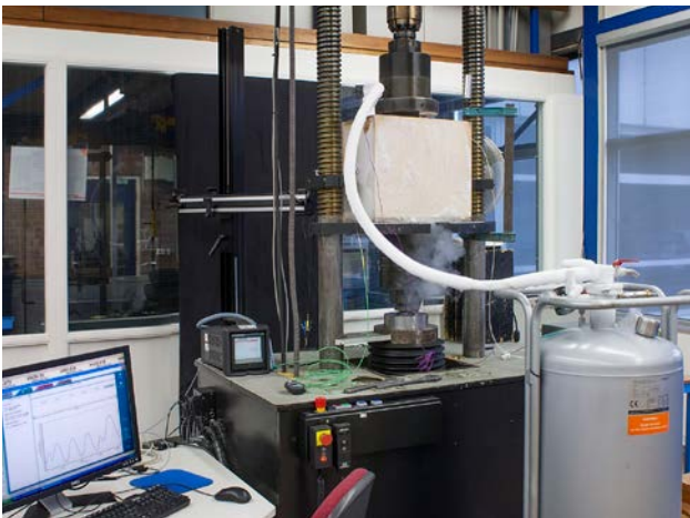
New approach of cooling of a fatigue test specimen: crack growth testing of Glare, 24/7 at -55°C.
