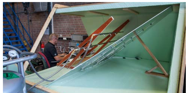
Next step; cross section of prototype setup to explore full-scale space structures testing at -180^{\circ}\text{C} .
