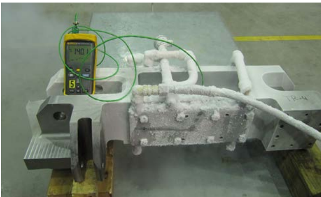
Thermal blocks, or heat sinks, to thermally insulate the test article from the test rig.
